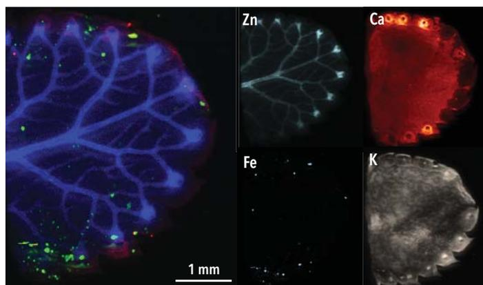
**Figure 2.** AttoMap Micro-XRF provides elemental imaging for multiple elements simultaneously. Left: tri-color composite of Zn (blue), Fe (green), and Ce (red). Right: individual channels for elements of interest. *Courtesy of Cerege, CNRS, Aix-Marseille University.*
